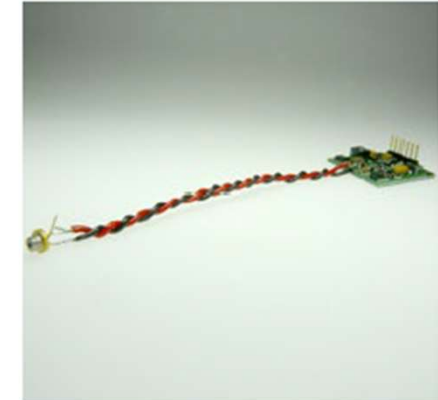
PLD connected by braided wires (length: 100 mm) Current rise time approx. >130 ns
