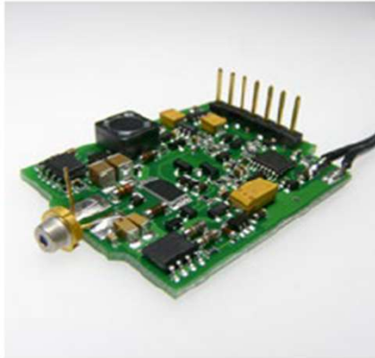
PLD directly connected to the driver Current rise time approx. 3.5 ns
