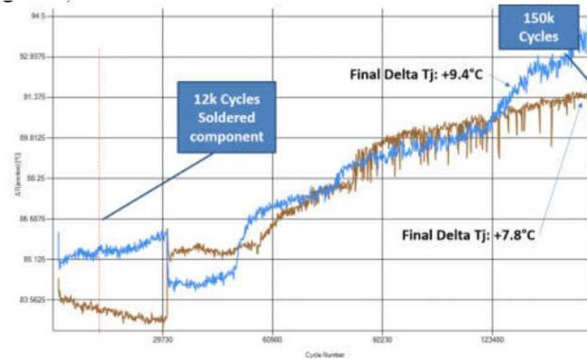
Fig.8: Delta T°C results after active power cycling test for sintered components, 2 worst cases presented. No failure arriving till 150k cycles. Minor increasing on the measurement is coming from grease “pumping out” phenomena.
