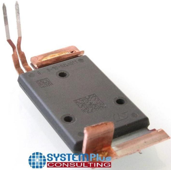
Automotive silicon carbide Power MOSFET 1200 V, 150 A
