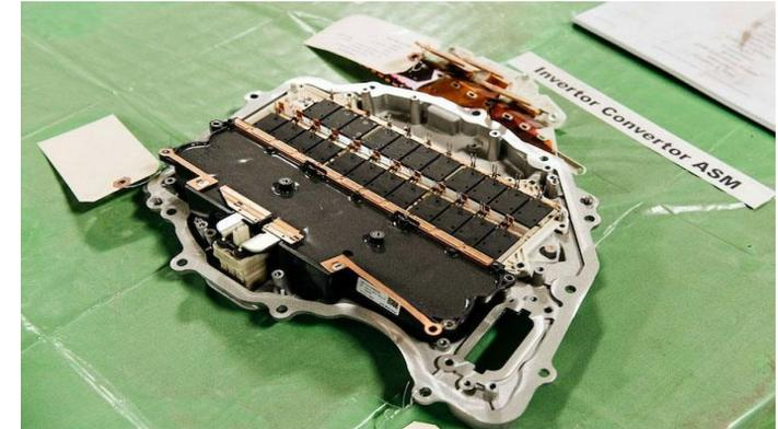
Model 3 inverter. Note two rows of rectangular devices
