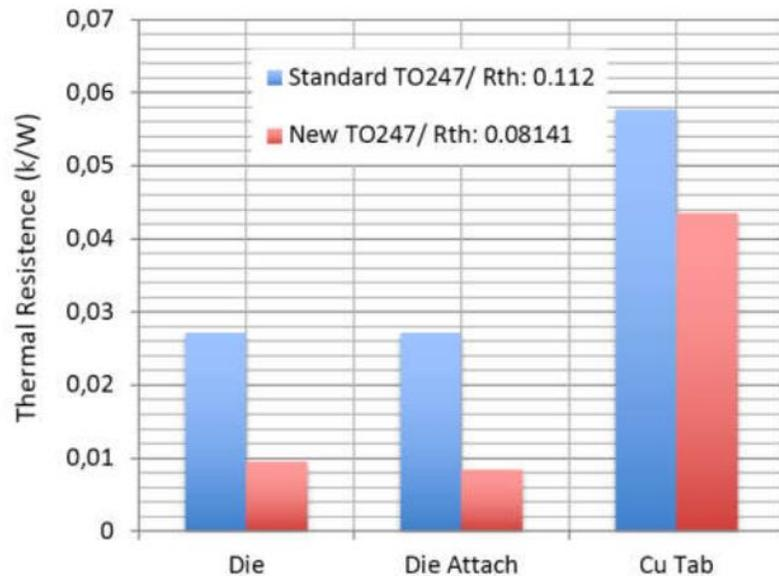
Fig.5: Thermal resistance comparison between classic TO247 and new component.
