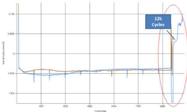
Fig.6: Vce continuous measurement during active power cycling test for soldered components, 2 best cases presented. Failure by 12k cycles, demonstrated by a spike on the Vce value, typical signature of wiring bond defect.
