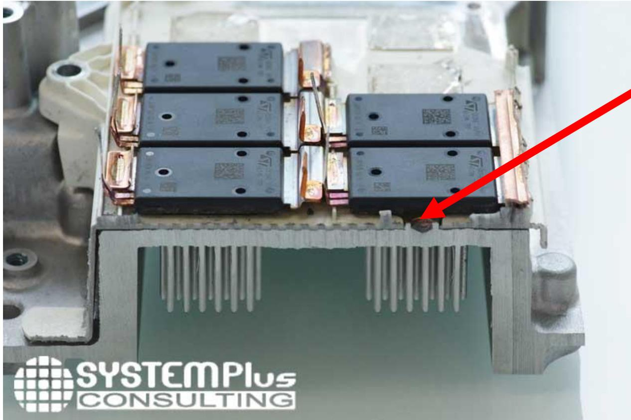
Sinter the package into the (inverter) housing.
