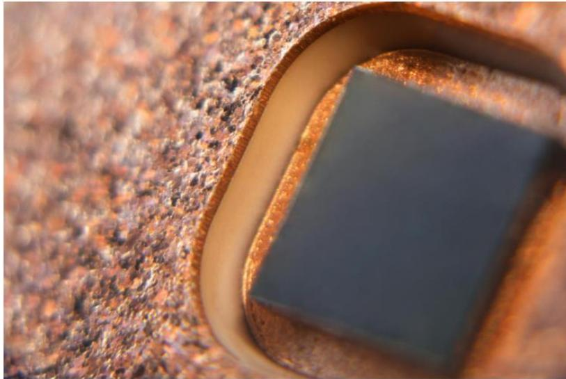
Close-up view of a wide-bandgap device embedded by the Ceramic Embedding technology.
