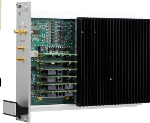
AWG18 (18bit / 300Msps AWG)
