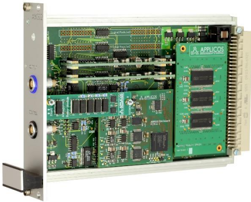
AWG22 (22bit / 2Msps AWG)
