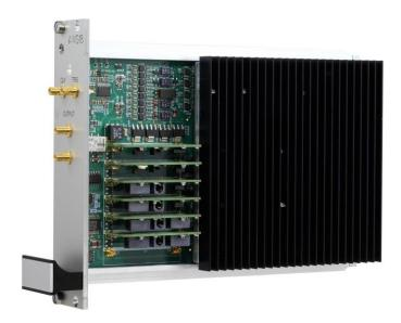
The module has 8 output ranges in steps of -3dB, which covers a wide range of Unit Under Test input voltages.
