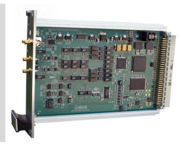
The AWG16 is a 16 bit Arbitrary Waveform Generator for high-speed / high resolution waveform generation. The fully differential signal path from the DAC all the way to the outputs ensures an exceptional high signal quality. Despite the emphasis on signal quality the AWG16 also has a very good DC accuracy.
